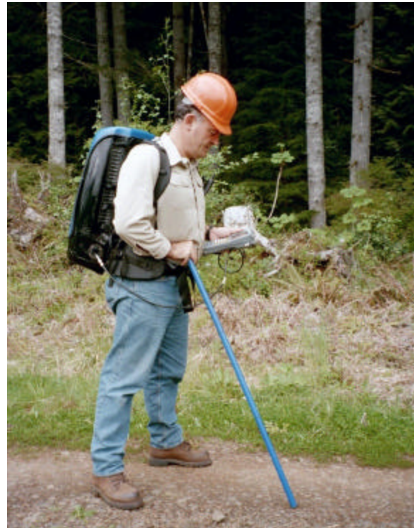
Figure 1. Applanix POS LS system is held steady in one position during a ZUPT.
