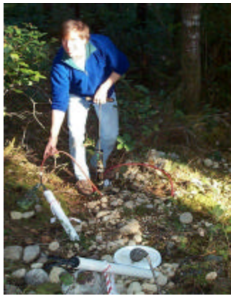
Dr. Adams is shown here collecting leachate from one of the 3 tube lysimeters installed at each plot in Doug-fir thinned plots. By pumping air into the tube, water is forced out of the other vacuum tube and into a collecting bottle (visible in the lower left of the photo). After collecting the soil water, the one-way valve is turned around and moved to the suction tube of the pump and the tube is recharged to -80 pps of pressure.
