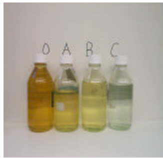
Lysimeters are installed at the surface (O horizon), into the A, B and C horizons. This photo shows the variation in color of the solutions that are extracted from the soil at variable depths. The bottle to the left labeled O was from the surface lysimeter (zero tension) and the bottle to the right was at a depth of 30-34 inches.
