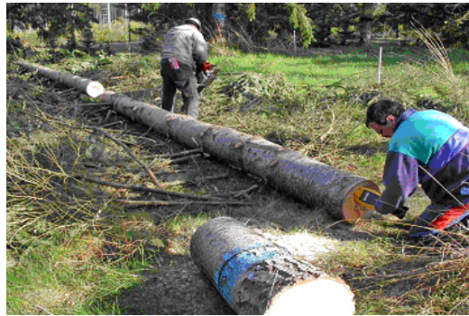
Randy Collier getting acoustic velocity of a log with the HM-200
