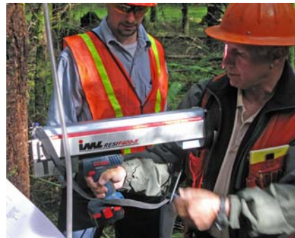
SMC Field Crew member Bob Gonyea demonstrates the Resistograph which measures resistance as a drill bit bores through a tree.
