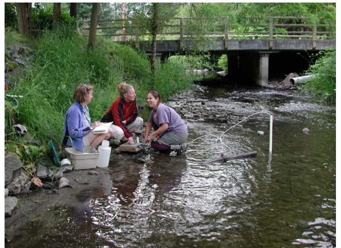
Testing water quality using in-stream wells.
